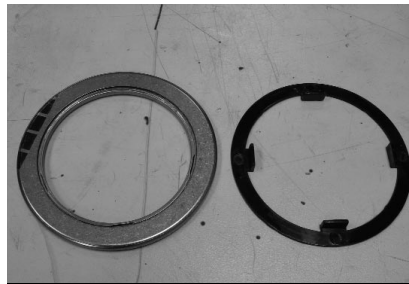
A durable Torrington roller bearing (left) replaces the flimsy plastic thrust washer (right) between the sun shell and the low reverse race. This is a high thrust area, and this plastic piece is one of the first items to wear—if it does, the race grinds into the sun shell.
