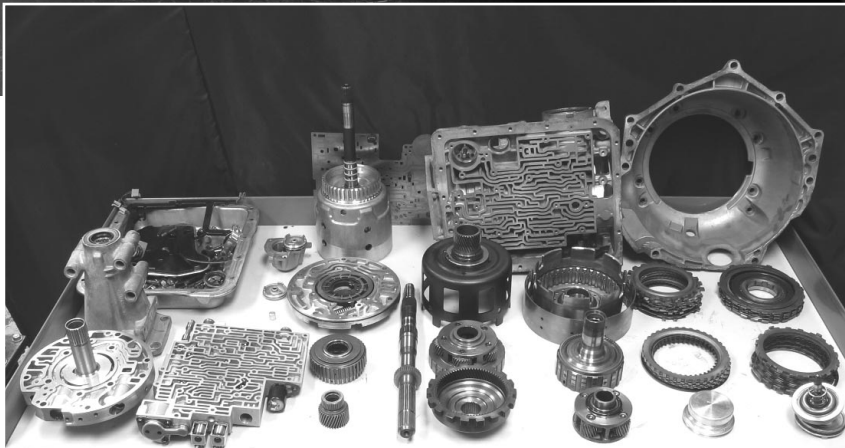
The completely disassembled tranny, Century Transmissions will turn your weak factory 4L60E into a 10-second-capable Street/Strip unit for $1875, barring any worn components or bad electronics.
