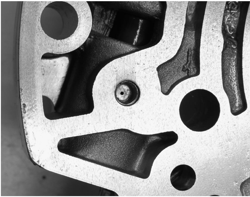
The TCC valve bleed orifice has been modified by installing an orifice cup plug in place of the two-piece OEM orifice. With the stock unit, the pin can sometimes fall through the seat, which will interfere with the lockup valve and possibly cause a non-lockup condition.
