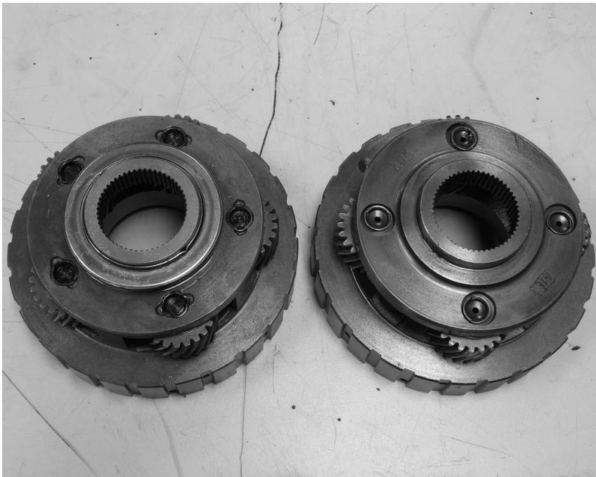
A strong trans needs strong internals. Here is the five-pinion Century Trans planetary on the left compared to a four-pinion GM planetary on the right. Century uses the five-pinion planetary to spread the load out on the carrier more, which makes it less likely to fail.
