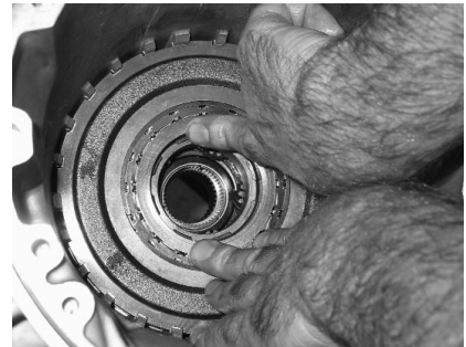
An anti-rattle clip is installed, and Ronnie pre-lubes the low/reverse sprag with a mixture of Mercon-III trans fluid and JB gear oil treatment.
