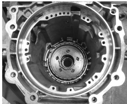
Ronnie Dorris, the head transmission tech at Century Automotive, begins the installation. After the factory ring goes in, the five-pin low/reverse planetary is lowered into place and connects to the splines of the output shaft.
