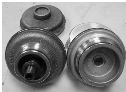
Here is the stock apply servo for second and fourth gear on the left, and a billet apply servo on the right. The billet unit has a larger apply area for a crisper band apply and 40 percent more holding power over a stock servo.
