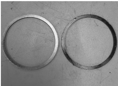
A cast GM rotor ring is on the left, with Century Trans' stronger hardened ring on the right. The hardened unit means less of a chance of the rotor vane breaking.
