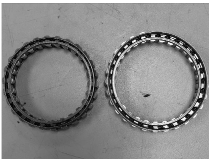
The input sprag, which is found inside the input drum, is upgraded from 26 segments to 29. This distributes the load from all four forward gears more evenly. The 26-segment sprag can slip the races, and when shifting to Third, this can cause a clutch-slipping effect.
