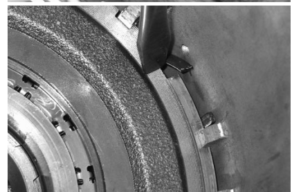
When installing the low/reverse sprag, the inner race should rotate clockwise to seat it. Next, the snap ring is installed, and Dorris uses a long-handled flat screwdriver to ensure that the ring is installed correctly. Finally, Ronnie uses compressed air to leak-check the reverse clutch operation.
