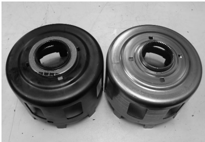
This shot shows an upgraded Century Trans Super Sun Shell on the left, a stock sun shell on the right. Century Trans has found that the thickness of the sun gear spline ring from GM can vary up to 30 thousandths, and these sun shells can crack behind even a totally stock motor! The Century shell is a GM part with a hardened sleeve used to prevent cracking around the sun gear splines. Its sleeve has to be custom-ground to each individual spline ring, then furnace brazed and black oxide coated.
