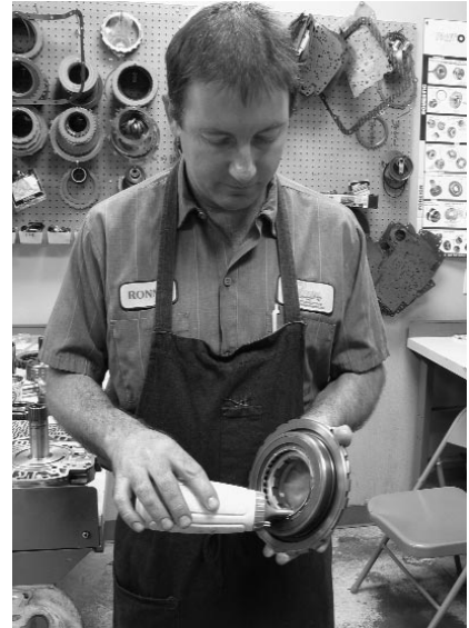
An anti-rattle clip is installed, and Ronnie pre-lubes the low/reverse sprag with a mixture of Mercon-III trans fluid and JB gear oil treatment.
