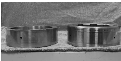
Century Trans modifies the factory low reverse inner sprag race (left) by grinding it down to make clearance for the rollerized Torrington bearing. This hardened steel unit is so hard that it can't be turned by a lathe.
